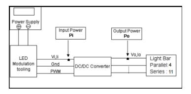
At 190 ~1kHz PWM control frequency, duty ratio range is restricted from 5% to 100%.
