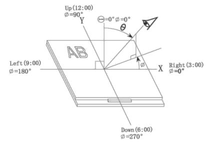
**Note 4:** Definition of contrast ratio Contrast measurements shall be made at viewing angle of  $\Theta = 0$  and at Victronix Tecenstar INT'L Co., LTD Tel:86-755-33265935 Email:sales@victronix-tech.com
